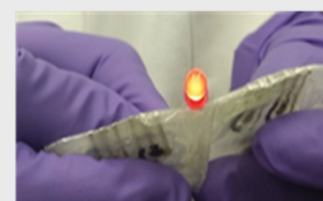
Demonstration of the performance of the tattoo battery under deformed conditions.
